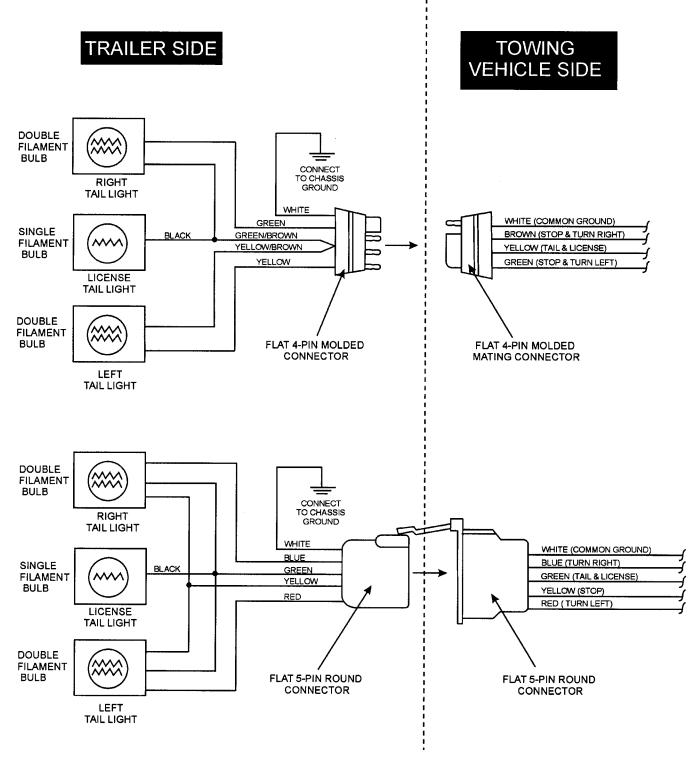
Figure 60. Trailer/Towing Vehicle Wiring Diagram
